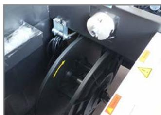
ALLOGGIO INTERNO BOBINA REGGIA
